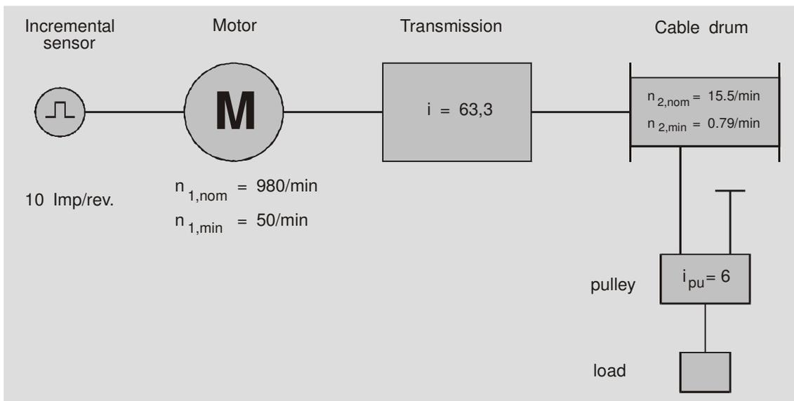
Fig. 7: Example of a lifting gear to be monitored
