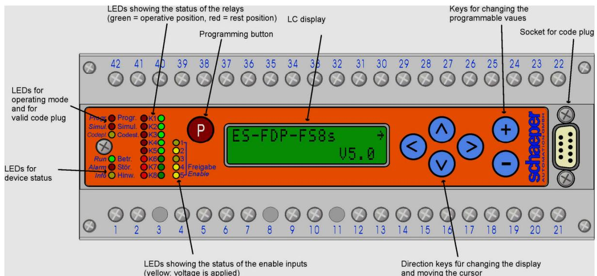
**Fig. 3:** Operating elements of the device
