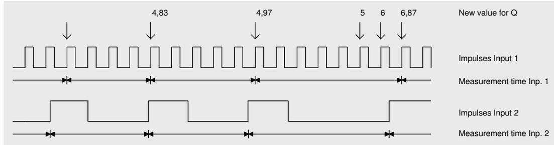
**Fig. 2:** Measurement times for the calculation of the quotients
